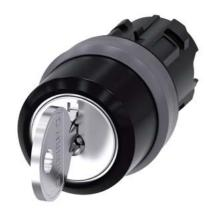
RONIS key-operated switch, 22 mm, round, plastic with metal front ring, lock number SB30, with 2 keys, 3 switch positions I-O-II, latching, actuating angle 2x45°, 10:30h/12h/13:30h, key removal O+I, possible special locks: SB31, 421, 455 Z=50-unit packaging
