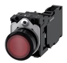
Illuminated pushbutton, 22 mm, round, plastic, red, pushbutton, flat, momentary contact type, with holder, 1 NO+1 NC, LED module with integrated LED 24 V AC/DC, screw terminal, with laser labeling, upper case
