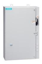
Non-reversing motor starter, Size 1, Three phase full voltage, Solid-state overload relay, OLR amp range 0.25-1A, 24VAC 50-60Hz coil, Combination type, 30A fusible disconnect, 30A/600V fuse clip, Enclosure NEMA type 4/12, Water/dust tight for outdoors, Extra-wide enclosure
