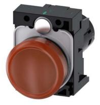
Indicator lights, compact, 22 mm, round, plastic, amber, lens, smooth, with holder, Operating voltage 110 V AC, screw terminal
