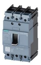
circuit breaker 3VA5 UL frame 125 breaking capacity class S 25kA @ 480 V 3-pole, line protection TM210, FTFM, In=60A overload protection Ir=60A fixed short-circuit protection Ii=10 x In UL489 SB (naval), 50 deg. cel. cable connection on both sides
