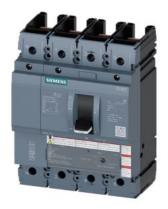
circuit breaker 3VA5 UL frame 250 breaking capacity class H 65kA @ 480V 4-pole, line protection TM230, FTAM, In=200A overload protection Ir=200A fixed short-circuit protection Ii=5...10 x In N conductor unprotected without connection
