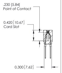
ACAD REFERENCE NO. 725-ENG MASTER 725 Series Ultra-Mate Card Edge Connector - Press Fit SEGAHON:3A:9A DRAWN: J.LEE Part Number: 725-038-545-201 CHECKED: DATE: SCALE: **EDAC INC** SHEET 1 OF 1 THESE DRAWINGS AND SPECIFICATIONS ARE THE PROPERTY OF EDAC INC.,AND TORONTO, ONTARIO SHALL NOT BE REPRODUCED, OR COPIED DRAWING NUMBER **ISSUE** CANADA OR USED AS THE BASIS FOR THE 725-ENG MASTER MANUFACTURE OR SALE OF APPARATUS YOUR CONNECTION TO QUALITY & SERVICE WITHOUT WRITTEN PERMISSION.
