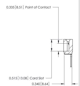
ACAD REFERENCE NO. 746 Series Ultra-Mate Card Edge Connector - Press Fit DRAWN: J.LEE Part Number: 746-024-545-101 CHECKED: **EDAC INC** SCALE: THESE DRAWINGS AND SPECIFICATIONS ARE THE PROPERTY OF EDAC INC.,AND TORONTO, ONTARIO SHALL NOT BE REPRODUCED, OR COPIED DRAWING NUMBER CANADA OR USED AS THE BASIS FOR THE 746-ENG MASTER MANUFACTURE OR SALE OF APPARATUS YOUR CONNECTION TO QUALITY & SERVICE WITHOUT WRITTEN PERMISSION.
