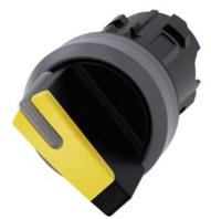
Selector switch, illuminable, 22 mm, round, plastic with metal front ring, yellow, selector switch, short, 2 switch positions O<I, momentary contact type, Actuating angle 45°, 10:30h/12h, Z=50-unit packaging
