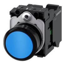
Pushbutton, 22 mm, round, plastic, blue, pushbutton, flat, momentary contact type, with holder 1 NO, spring-type terminal, with laser labeling, upper case
