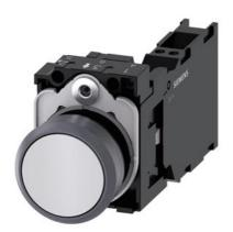
Pushbutton, 22 mm, round, plastic with metal front ring, white, pushbutton, flat, momentary contact type, with holder, 1 NO+1 NC, spring-type terminal, with laser labeling, lower case
