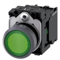
Illuminated pushbutton, 22 mm, round, plastic with metal front ring, green, pushbutton, flat, momentary contact type, with holder, 1NO, LED module with integrated LED 24 V AC/DC, screw terminal, Z=20-unit packaging
