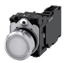
Illuminated pushbutton, 22 mm, round, Metal, shiny, white, pushbutton, flat, momentary contact type, with holder, 1 NO+1 NC, LED module with integrated LED 230 V AC, screw terminal, with laser labeling, inscription or symbol Customer-specific selection with SIRIUS ACT configurator (CIN)
