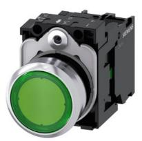
Illuminated pushbutton, 22 mm, round, Metal, shiny, green, pushbutton, flat, momentary contact type, with holder, 1NO, LED module with integrated LED 230 V AC, screw terminal, with laser labeling, upper case and lower case, always upper case at the beginning of the word
