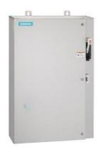
Non-reversing motor starter Size 1 Three phase full voltage Solid-state overload relay OLRelay amp range 10-40a Combination type 60Amp non-fused disconnect Encl NEMA type 4X 316 S-steel Water/dust tight non-corrosive Extra-wide enclosure
