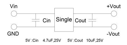
To make sure the product work at perfect operation status with full loading external capacitor is necessary and it is recommended to use high frequency low resistance electrolytic capacitor.
