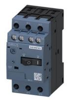
Circuit breaker size S00 for motor protection, CLASS 10 A-release 7...10 A N release 130 A Screw terminal Standard switching capacity with transverse auxiliary switch 1 NO+1 NC  $\,$
