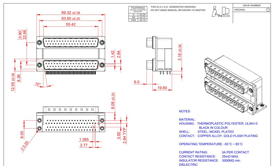
WITHSTANDING VOLTAGE: 1000V AC rms
