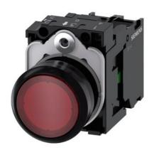
Illuminated pushbutton, 22 mm, round, plastic, red, pushbutton, flat, momentary contact type, with holder, 1NO, LED module with integrated LED 24 V AC/DC, screw terminal, Z=20-unit packaging
