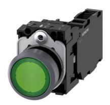
Illuminated pushbutton, 22 mm, round, plastic with metal front ring, green, pushbutton, flat, momentary contact type, with holder, 1 NO+1 NC, LED module with integrated LED 24 V AC/DC, screw terminal, with laser labeling, inscription or symbol Customer-specific selection with SIRIUS ACT configurator (CIN)
