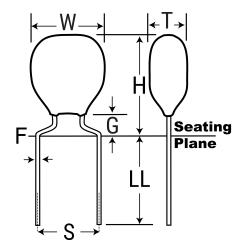
**General Information** Series T368 Dielectric MnO2 Tantalum Style Radial Description Radial, Solid Tantalum, Conformal, Retangular Anode Features **Rectangular Anode** RoHS Yes Termination Tin AEC-Q200 No Notes Longest Lead Is Positive.
