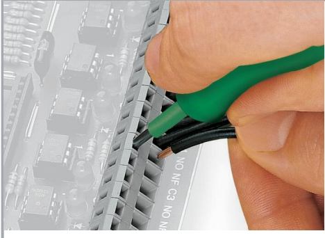
Inserting a conductor via 3.5 mm screwdriver.
