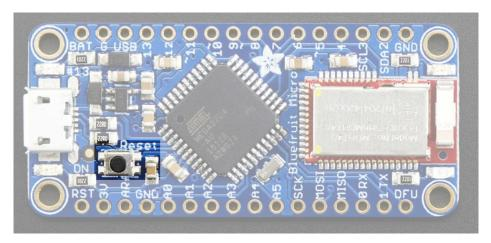
To the right is a small tactile switch. This is the reset button for the ATmega32u4. You can use this to reset the microcontroller and/or push it into bootloader mode if the bootloader gets 'stuck' during programming
