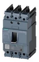
circuit breaker 3VA5 UL frame 125 breaking capacity class H 65kA @ 480V 3-pole, line protection TM230, FTAM, In=20A overload protection Ir=20A fixed short-circuit protection Ii=7.5...15 x In UL 489 SB (naval), 50° C without connection
