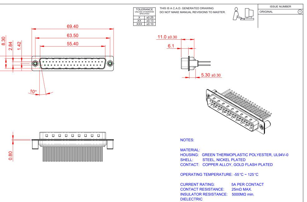
WITHSTANDING VOLTAGE: 1000V AC rms
