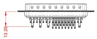
10A (CURRENT) POWER/CO-AX CONTACT RATING: (IF PRESENT) SIGNAL CONTACT CURRENT RATING: 5A PER CONTACT SIGNAL CONTACT RESISTANCE:  $10m\Omega$  MAX. INSULATOR RESISTANCE: 5000MΩ min. DIELECTRIC
