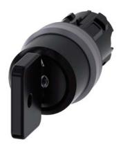
Key-operated switch O.M.R, 22 mm, round, plastic with metal front ring, lock number 73034, black, with 2 keys, 3 switch positions I>O<II, momentary contact type, actuating angle 2x45°, 10:30h/12h/13:30h, key removal O, with laser labeling, lower case
