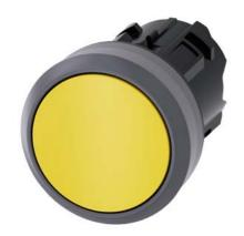
Pushbutton, 22 mm, round, plastic with metal front ring, yellow, pushbutton, flat, latching, Push-to-release mechanism, with laser labeling, upper case
