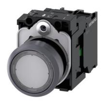
Illuminated pushbutton, 22 mm, round, plastic with metal front ring, clear, pushbutton, flat, momentary contact type, with holder, 1NO, LED module with integrated LED 24 V AC/DC, screw terminal, with laser labeling, upper case and lower case, always upper case at beginning of line
