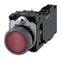
Illuminated pushbutton, 22 mm, round, plastic with metal front ring, red, pushbutton, flat, momentary contact type, with holder, 1 NO+1 NC, LED module with integrated LED 24 V AC/DC, screw terminal, with laser labeling, upper case and lower case, Always upper case at the beginning of the word
