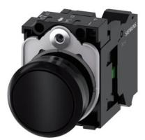
Pushbutton, 22 mm, round, plastic, black, pushbutton, flat, momentary contact type, with holder 1 NO, spring-type terminal, with laser labeling, upper case
