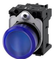
Indicator lights, 22 mm, round, plastic, blue, lens, smooth, with holder, LED module, with integrated LED 24 V AC/DC, screw terminal, with laser labeling, lower case
