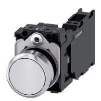
Pushbutton, 22 mm, round, metal, shiny, white, pushbutton, flat, momentary contact type, with holder, 1 NO+1 NC, spring-type terminal, Z=20-unit packaging
