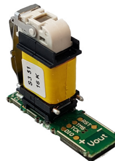
Figure 8. Switch Reference Design without the Wings
