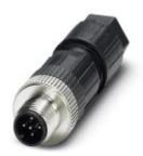
Connector, 5-position, Plug straight M12, A-coded, Spring-cage connection, knurl material: Zinc die-cast, nickel-plated, external cable diameter 4 mm ... 8 mm
