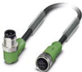
Sensor/actuator cable, 3-position, Variable cable type, Plug angled M12, A-coded, on Socket straight M12, A-coded, cable length: Free input (0.2 ... 40.0 m)
