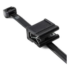
Low-profile clip attaches easily to plastic and metal edges as thin as 0.5 mm and up to 2.5 mm without the need for a mounting hole. Two designs allow bundles to be secured parallel or vertical to surface edges.
