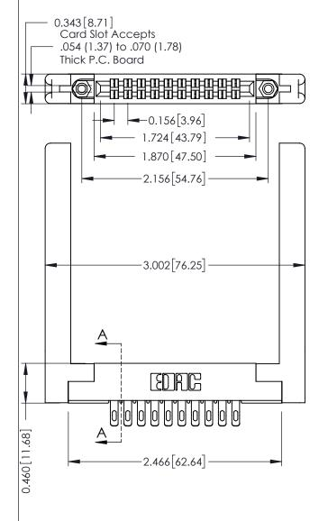
A-A0.295 [7.49] Card Slot **ECTION** 0.090[2.29] Point of Contact 305 ENG MASTER 305 / 315 / 355 Card Edge Connector
