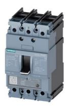
circuit breaker 3VA5 UL frame 125 breaking capacity class M 35kA @ 480 V 3-pole, line protection TM230, FTAM, In=20A overload protection Ir=20A fixed short-circuit protection li=7.5...15 x In cable connection on both sides
