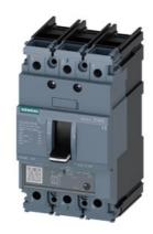
circuit breaker 3VA5 UL frame 125 breaking capacity class M 35kA @ 480 V 3-pole, line protection TM230, FTAM, In=90A overload protection Ir=90A fixed short-circuit protection Ii=5...10 x In UL489 SB (naval), 50 deg. cel. nut keeper kit on both sides
