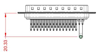
POWER/CO-AX CONTACT RATING:20A (CURRENT)(IF PRESENT)SIGNAL CONTACT CURRENT RATING:5A PER CONTACTSIGNAL CONTACT RESISTANCE:10mΩ MAX.INSULATOR RESISTANCE:5000MΩ min.
