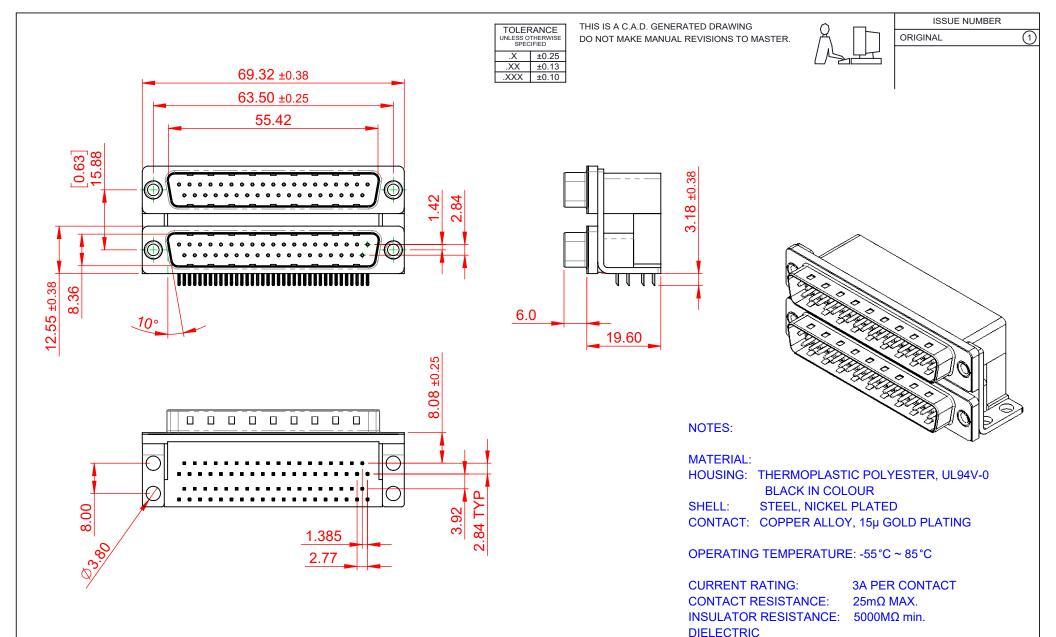
WITHSTANDING VOLTAGE: 1000V AC rms
