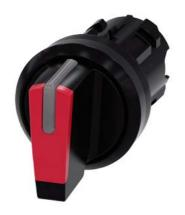
Selector switch, illuminable, 22 mm, round, plastic, red, selector switch, short, 3 switch positions I-O-II, latching, actuating angle  $2x45^{\circ}$ , 10:30h/12h/13:30h Z=50-unit packaging
