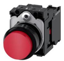
Pushbutton, 22 mm, round, plastic, red, pushbutton, raised, momentary contact type, with holder 1 NC, screw terminal, with laser labeling, upper case and lower case, always upper case at beginning of line
