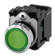
Illuminated pushbutton, 22 mm, round, metal, shiny, green, pushbutton, flat, momentary contact type, with holder, 1NO, LED module with integrated LED 110 V AC, spring-type terminal, with laser labeling, upper case and lower case, always upper case at beginning of line
