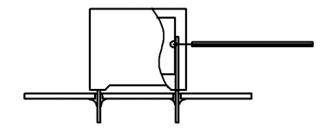
Temperature monitored inside the capacitor.
