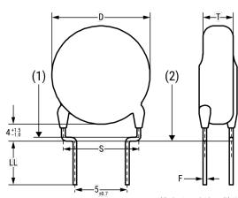
Coating on lead shall not extend below this line. (2) - Point of support on printed cardboard.
