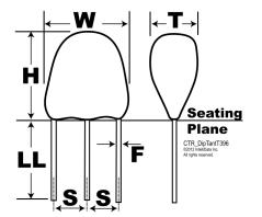
**General Information** Series T396 Dielectric MnO2 Tantalum Style **Radial Three Lead** Radial, Solid Tantalum, Three Leaded Description RoHS Yes Termination Tin AEC-Q200 No Construction Conformal Notes Longest Lead Is Positive.
