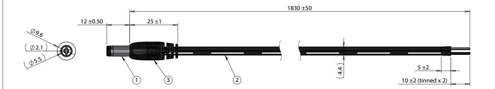
**Notes:** Functionally equivalent components may be substituted Cable rated for 48 V, 8.5A
