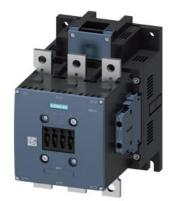
Contactor, AC-1, 400 A/690 V/40  $^\circ\text{C},$  S10, 3-pole, 440-480 V AC/DC, with varistor, 2 NO+2 NC, Connection rail/ screw terminal
